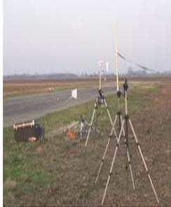
Flight-line equipment used to measure spray pattern
